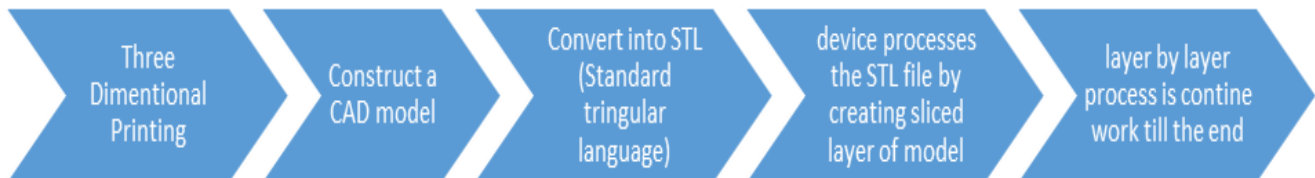
Fig. 2. 3D Printing Technique Basic Steps.
